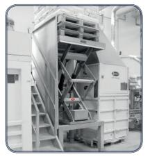
Lifting tables in mixed materials can be made e.g. galvanized scissor and bottom frame and stainless steel platform.
