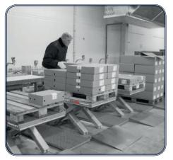
The tables are corrosion proof and resistant to the rugged conditions and use of aggressive cleaning products in e.g. the food industry.
